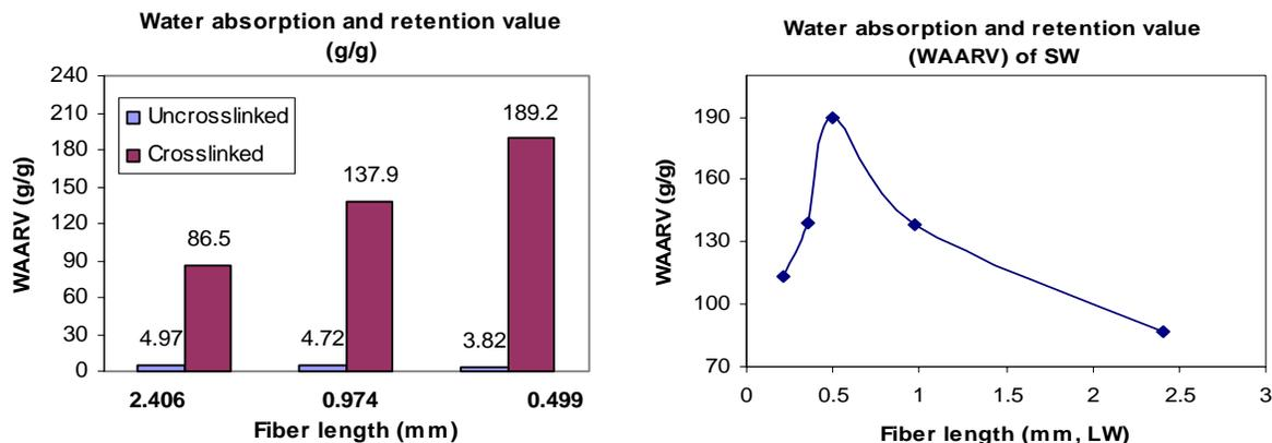
**Figure 1:** Water absorbency value of crosslinked ECF softwood kraft pulp. Water absorbency determined by water retained after centrifuging.
