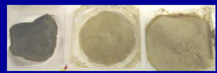
Air dried sludge from linerboard mills Left Rome GA, Middle Pine Hill AL, Right Springfield OR
