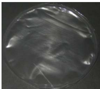
PLA-PBS-MCC nanocomposite film
