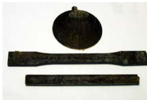
Figure 1. Picture of Recently Developed Kraft Pulp-Nylon 6 Post Consumer Carpet Composite Prepared by Injection Molding.
