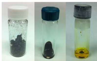
Figure 2. Pyrolysis products, char (left), heavy oil (middle) and light oil (right).
