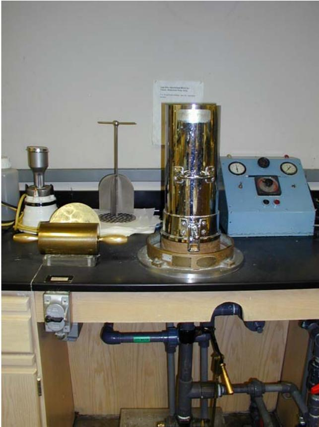
Figure 4. Handsheet making apparatus.
