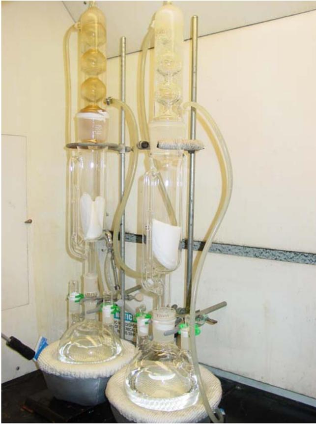
Figure 4. Soxhlet extraction apparatus.
