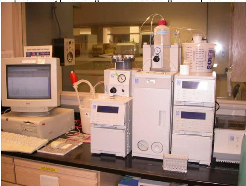
Figure 1. Photograph of high performance anion-exchange chromatography with pulsed amperometric detection (HPAEC-PAD).
