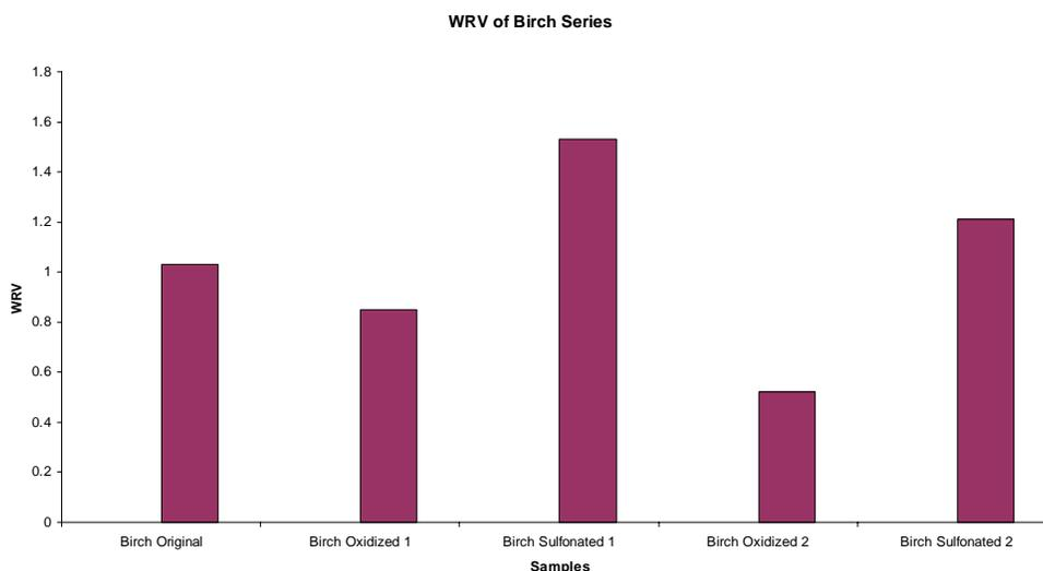
Figure 1. Water retention values (WRVs) of oxidized and sulfonated ECF bleached HW kraft pulp.
