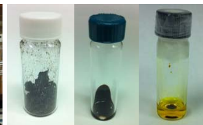
Figure 2. Products of pyrolysis, char (left), heavy oil (middle) and light oil (right).
