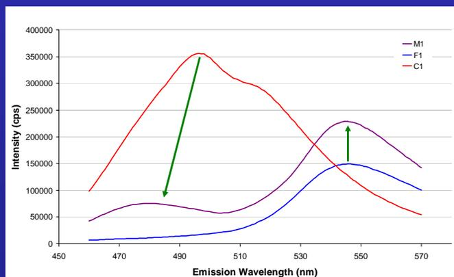
Figure 3 – Emission spectra of viscose sheets containing fluorescein dyed fibers (F1), coumarin dyed fibers (C1), and a mixture (M1).
