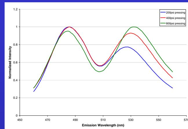
Figure 4 – Normalized emission spectra of viscose sheets wet pressed to different level containing both fluorescein dyed and coumarin dyed fibers.
