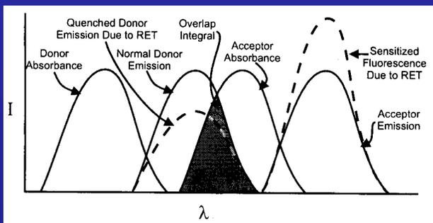
Figure 1 – Fluorescence resonance energy transfer [Herman. *Fluorescence Microscopy, 2<sup>nd</sup> Edition*. 1998].
