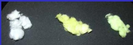
Figure 2 – Viscose fibers: Un-dyed (left), fluorescein dyed (center), and coumarin dyed (right).
